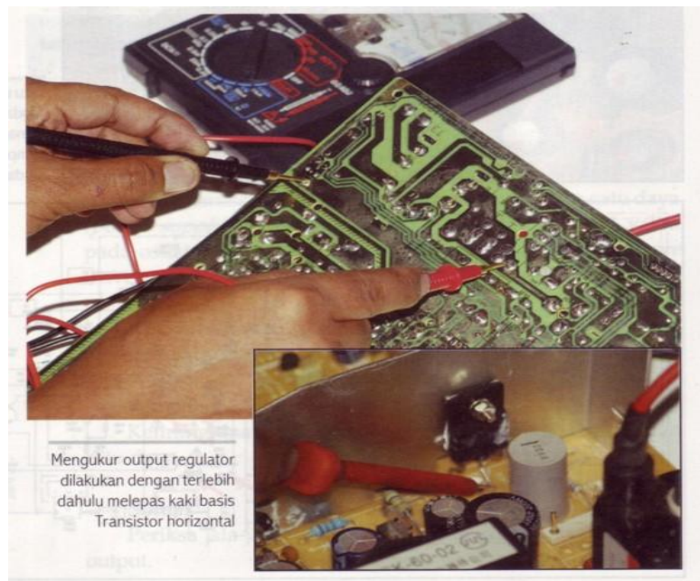
Gambar 19. Mengukur Output Regulator
